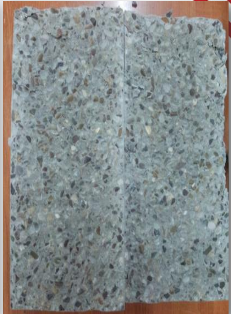
Figure (20) Splitting Tensile Strength Test
