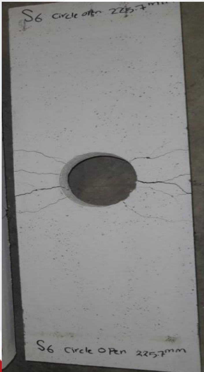
Figure (4 2 ) Crack pattern of specimen S6.
