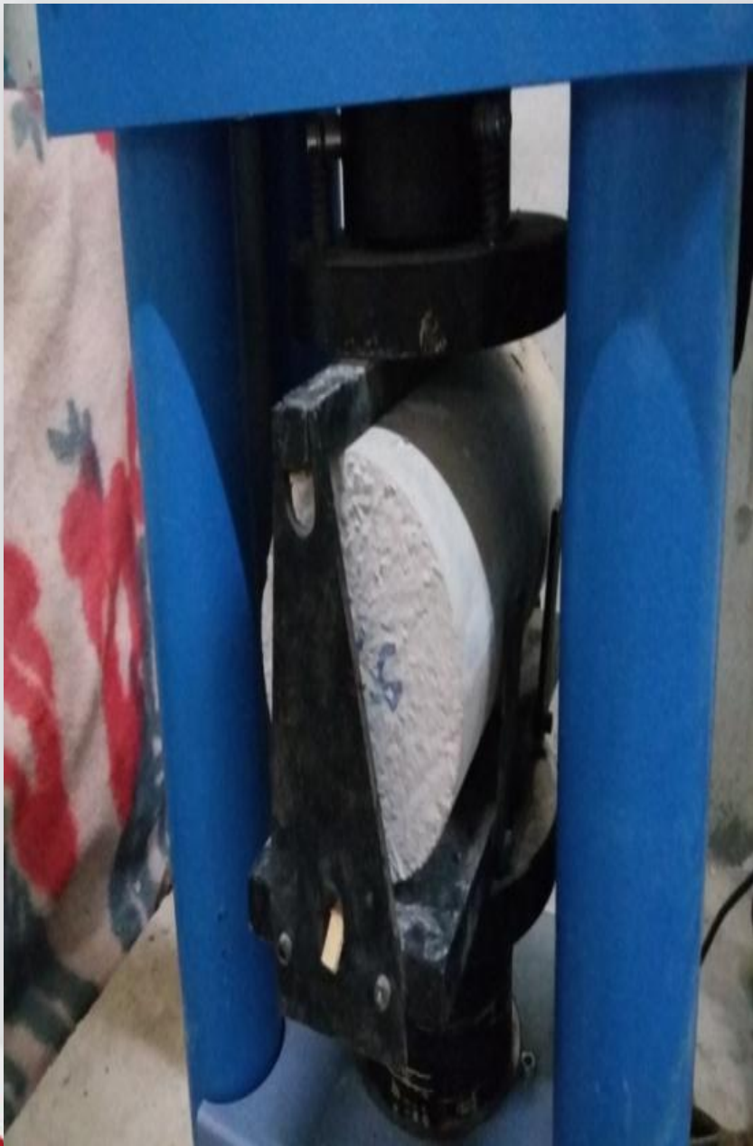
Figure (20) Splitting Tensile Strength Test
