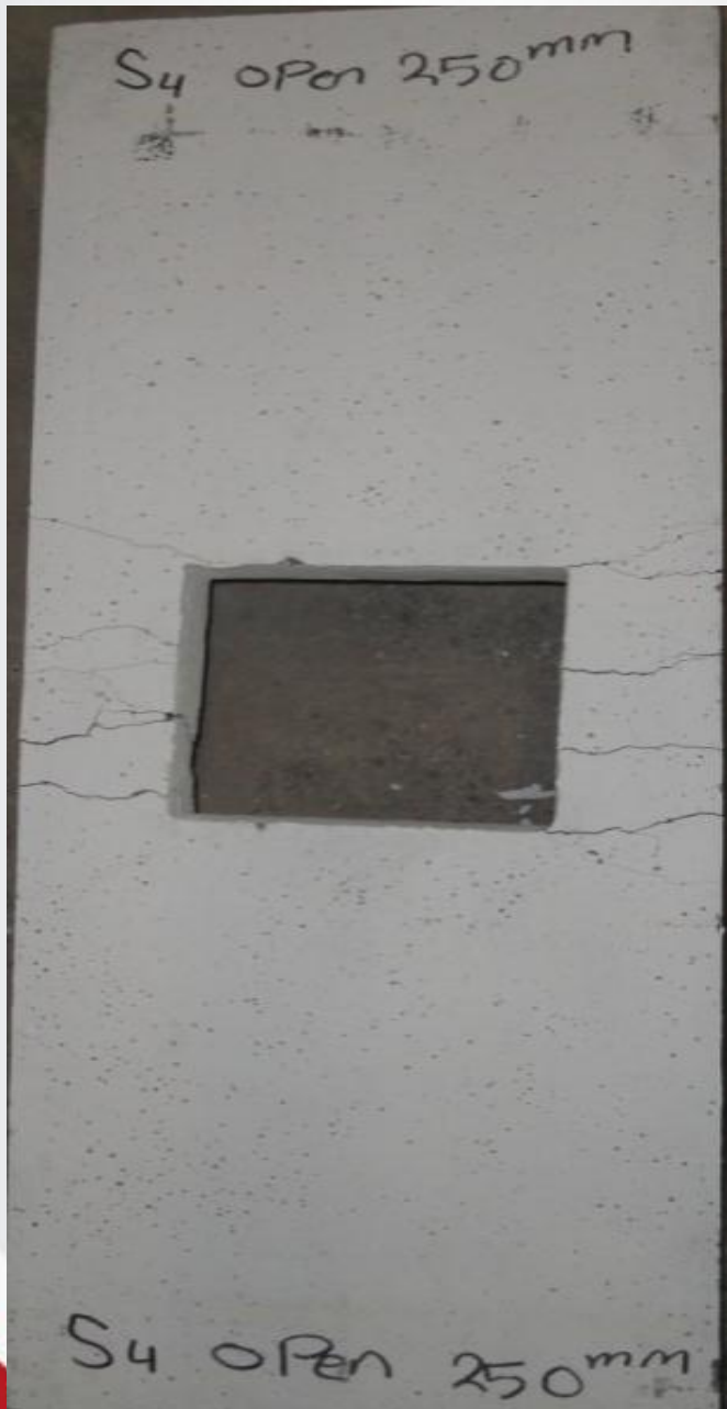
Figure (3 ^ ) Crack pattern of specimen S4.
