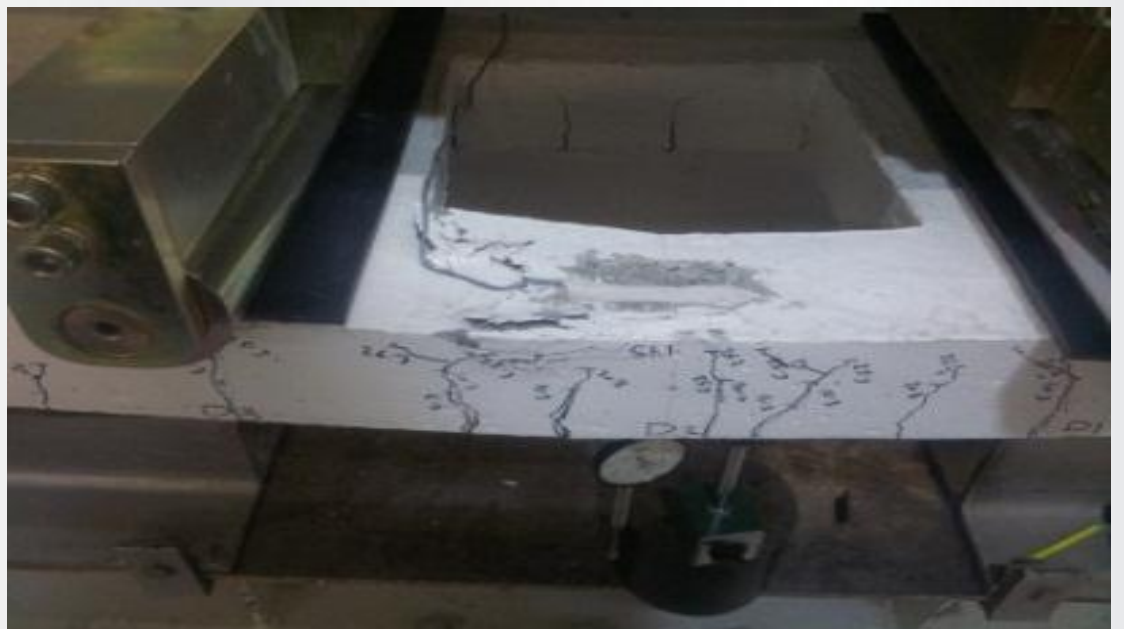
Figure (3 ^ ) Crack pattern of specimen S4.
