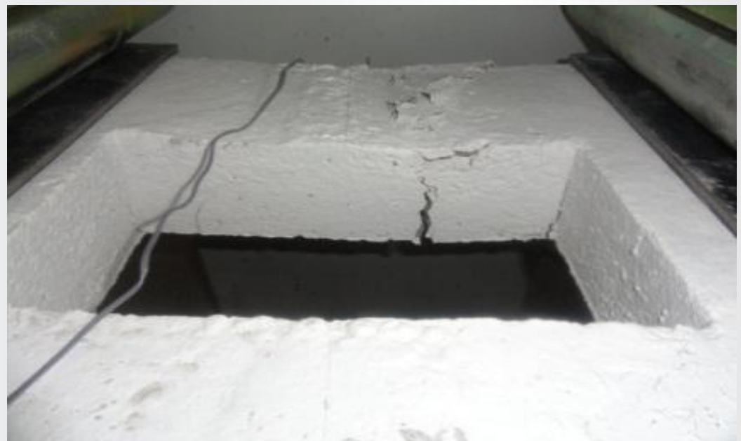
Figure (4.0) Crack pattern of specimen S5.
