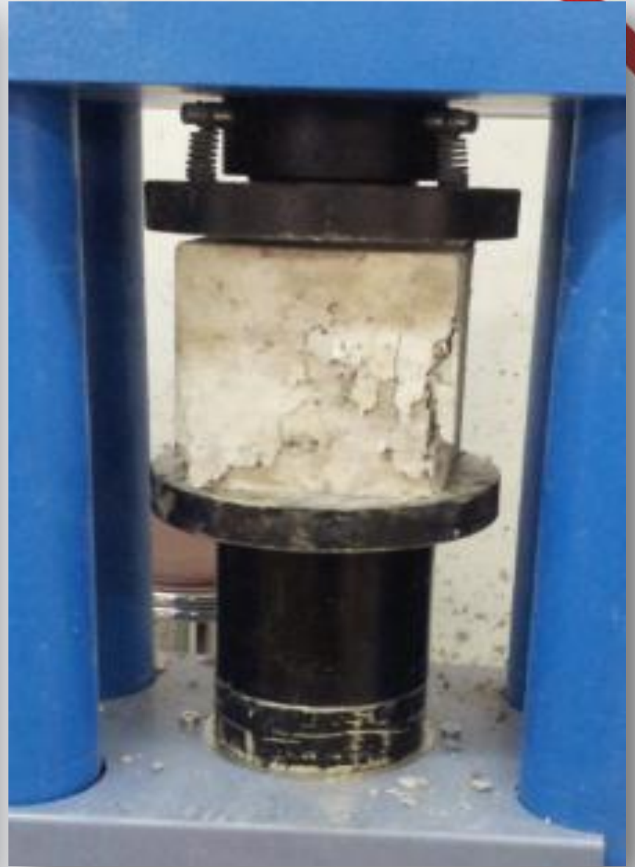
Figure (19) Compressive Strength Test
