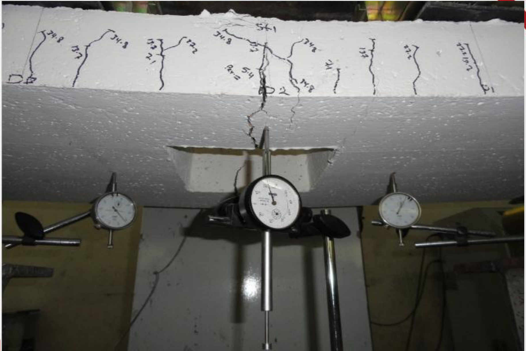
Figure (2 9 ) Dial Gauge Position.
