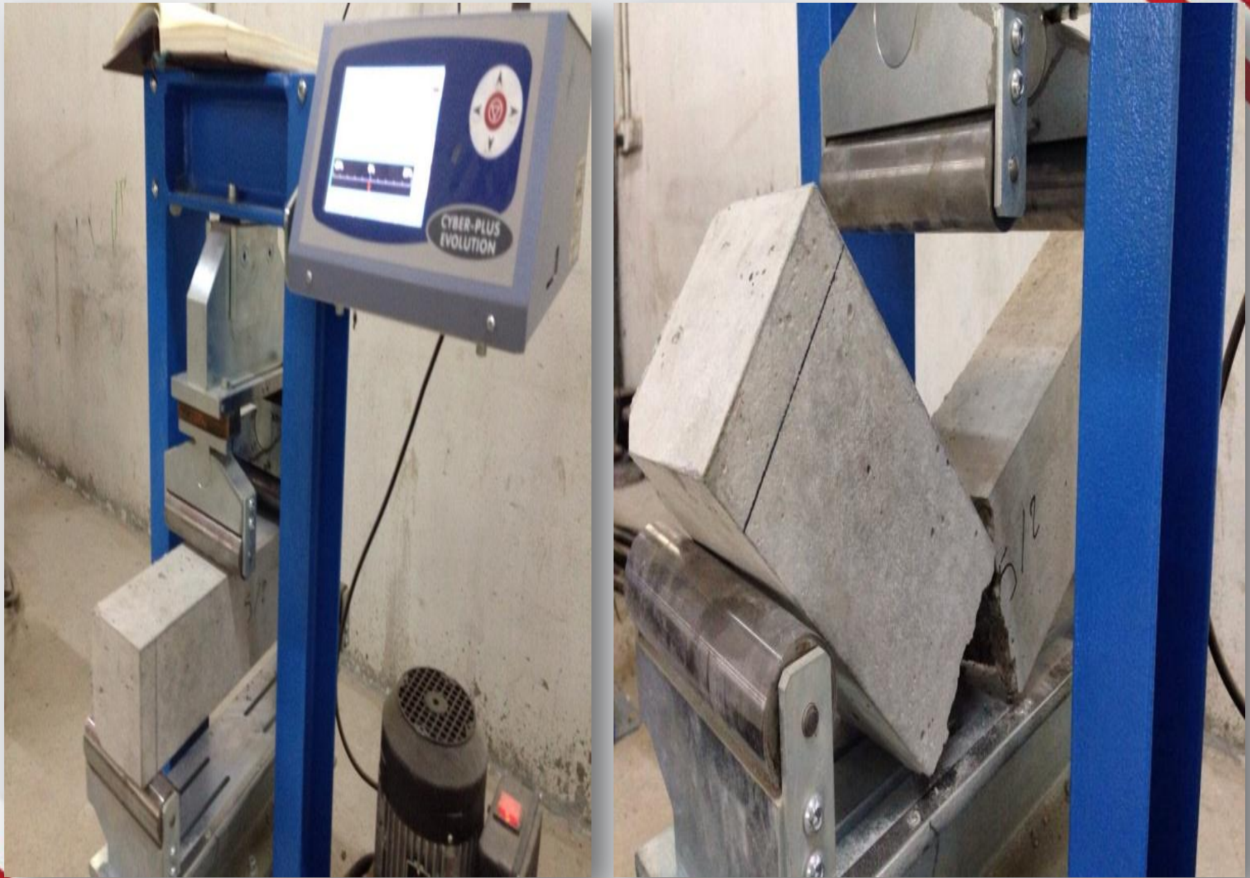
Figure (21) Flexural Strength Test
