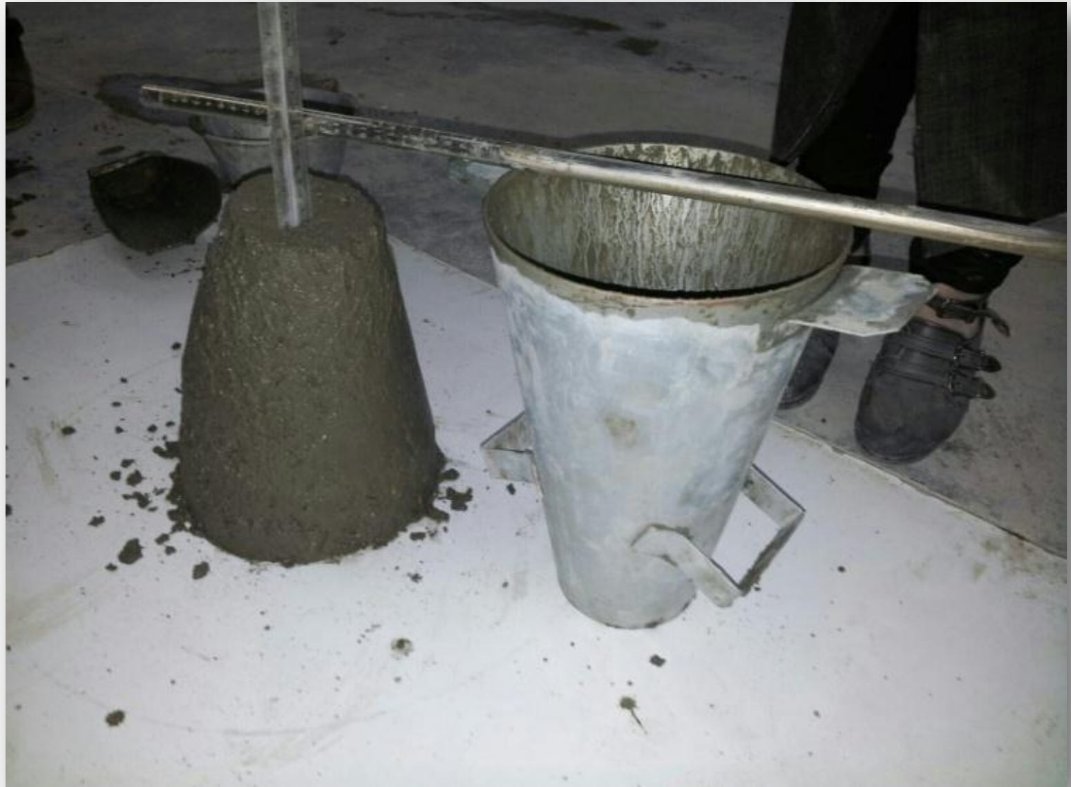
Figure (1۳) Slump Tests
