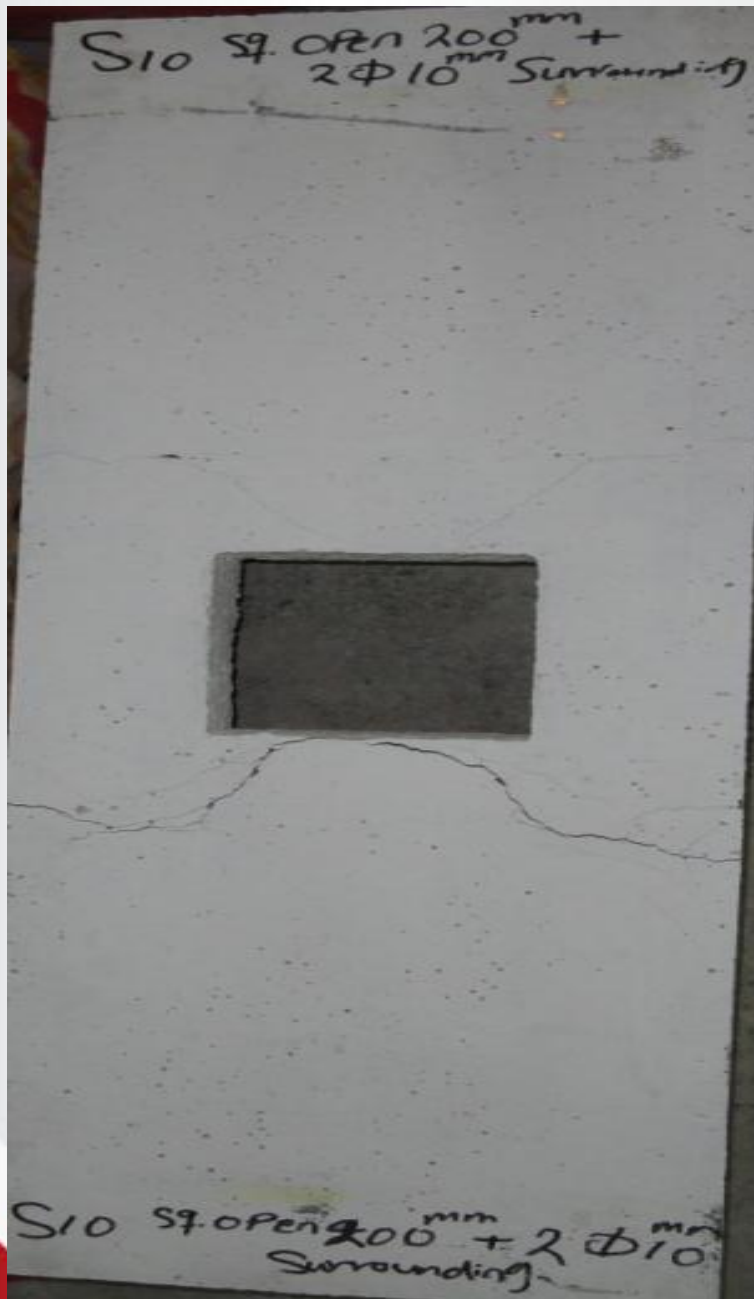
Figure (••) Crack pattern for S10.
