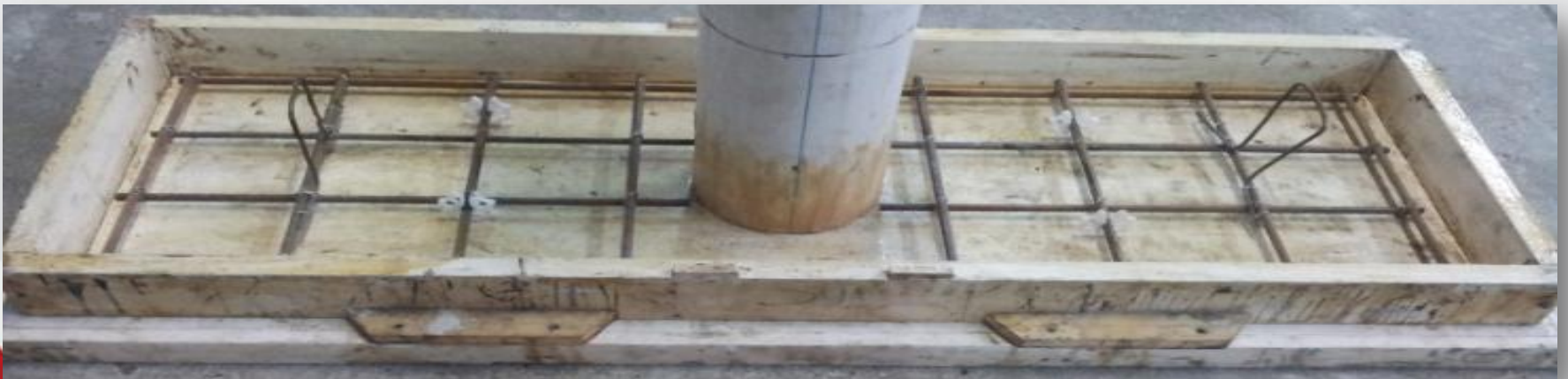
Figure (٦) group2 slabs reinforcement details.
