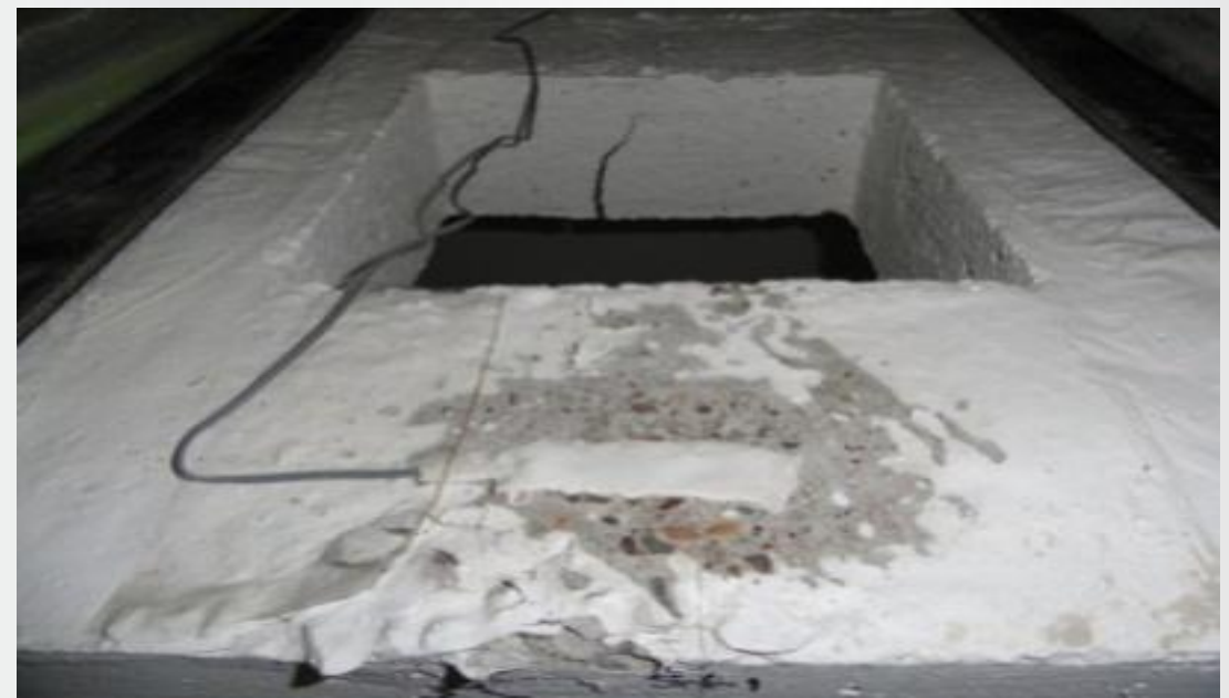
Figure (4 th ) Crack pattern of specimen S8.
