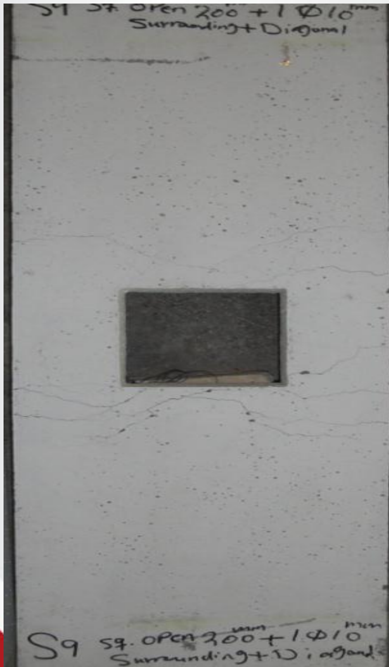
Figure (4 ^ ) Crack pattern of specimen S9.
