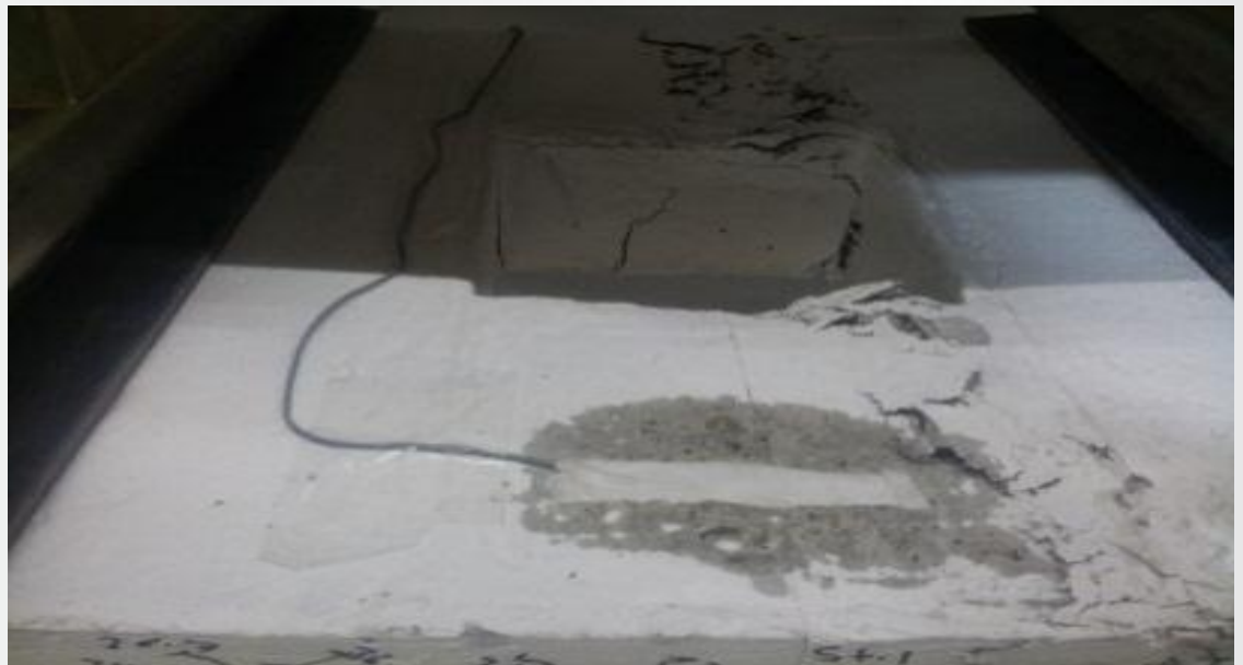
Figure (3 rd ) Crack pattern of specimen S3.
