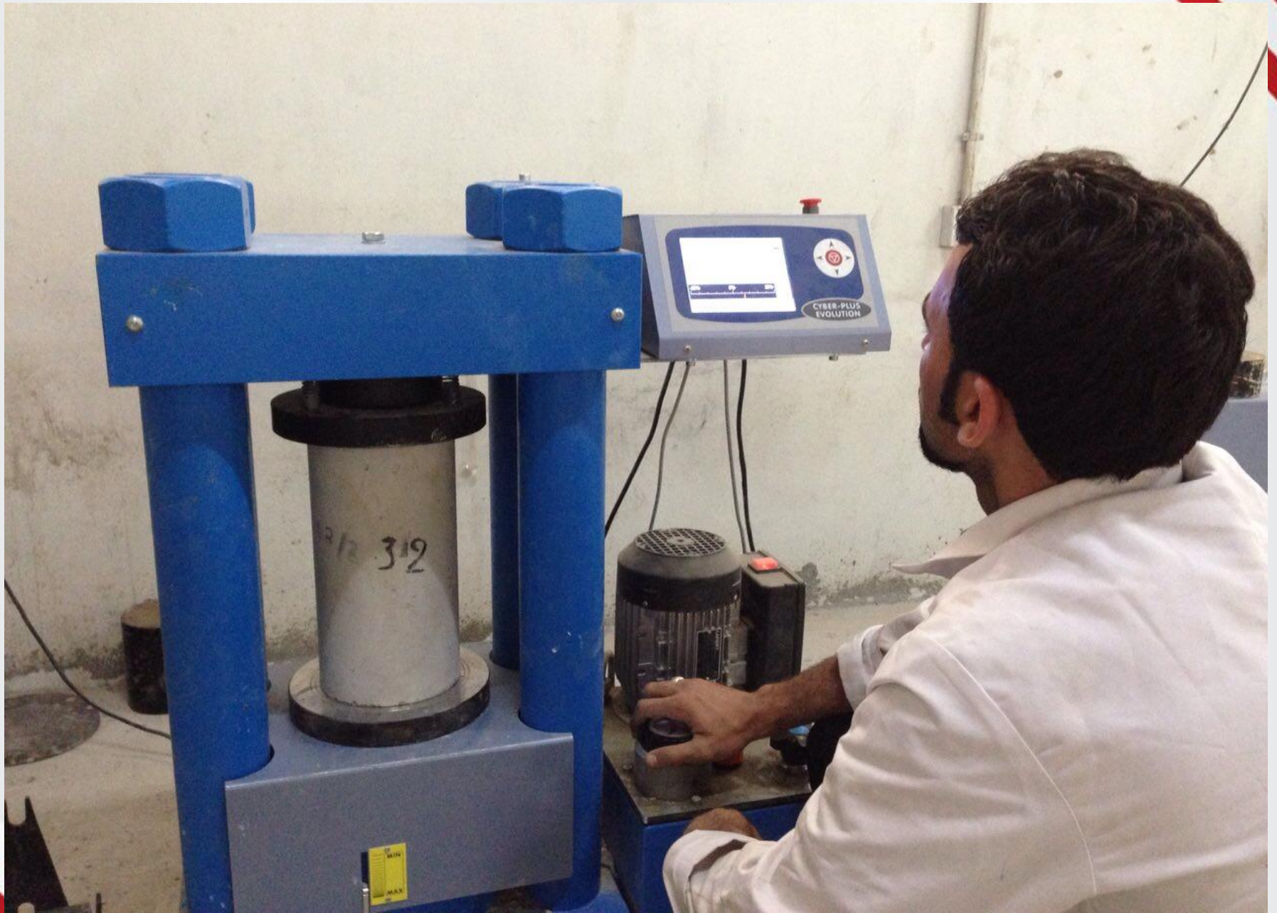
Figure (1 ^ ) Compressive Strength Test
