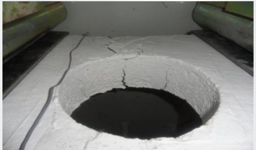
Figure (4 2 ) Crack pattern of specimen S6.
