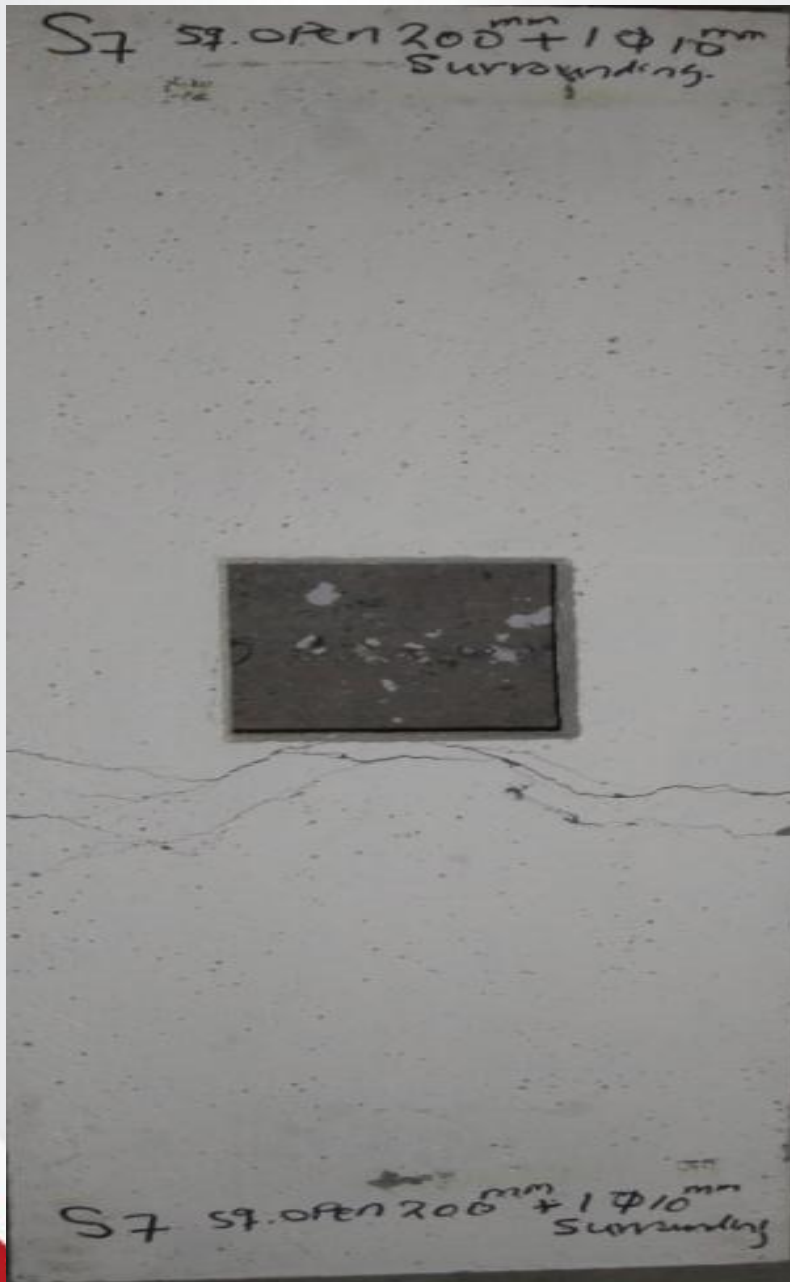
Figure (4 z ) Crack pattern for S7.
