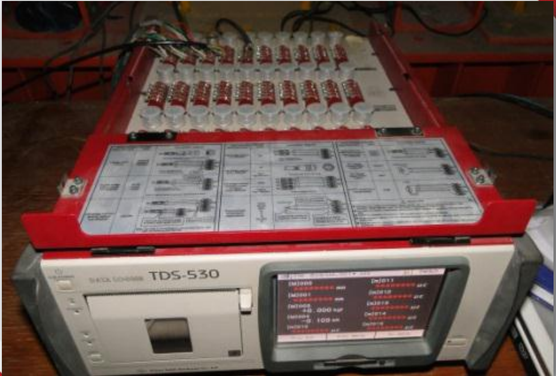
Figure (2 v ) Data Logger TDS-530.
