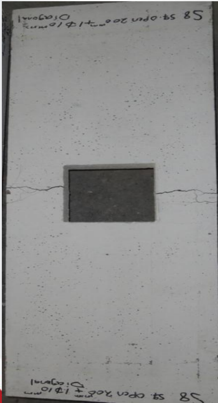
Figure (4 th ) Crack pattern of specimen S8.
