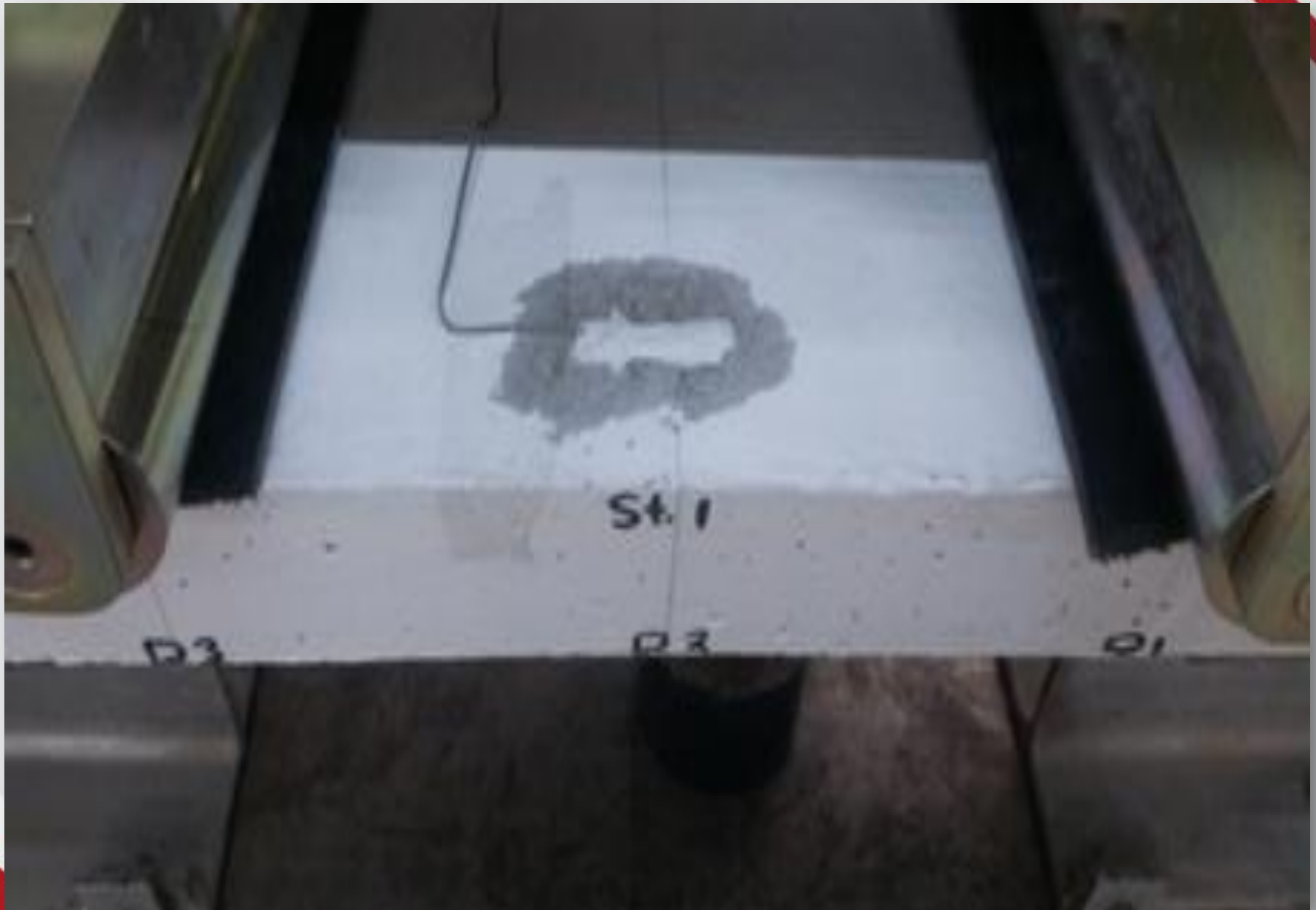
Figure (26) Strain Gauges Arrangement.
